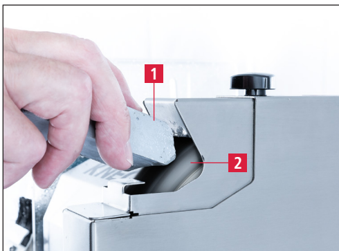
Figure 7-4 Applying the polishing paste
