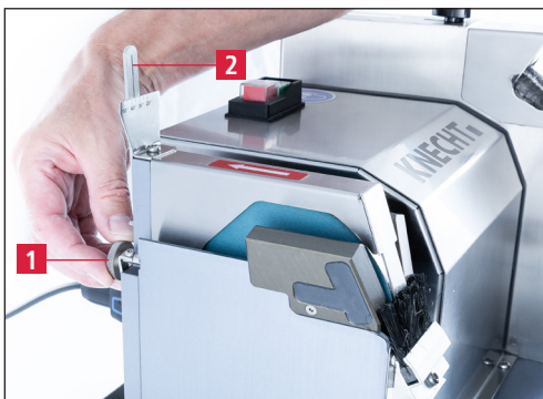
Figure 7-1 Adjusting the grinding angle
