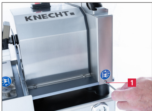
Figure 7-11 Loosening the polishing disk cover
