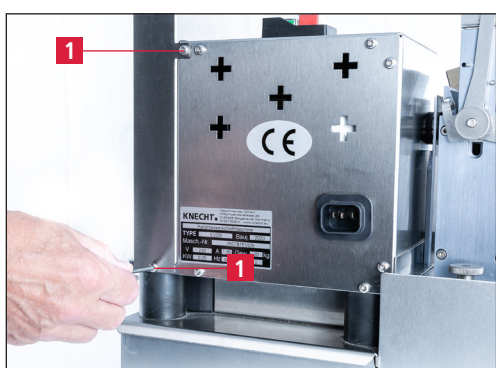
Figure 7-10 Loosening the polishing disk cover
