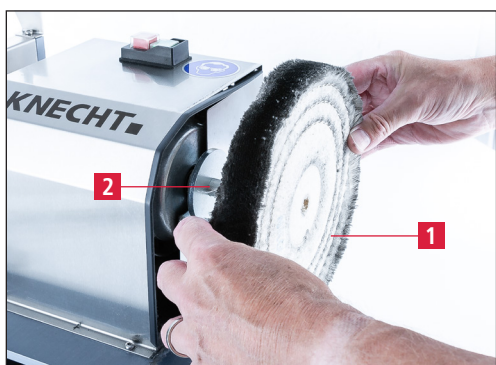
Figure 7-14 Replacing the polishing disk
