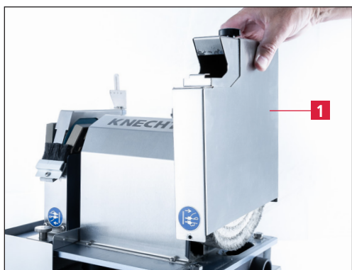
Figure 7-12 Removing the polishing disk cover
